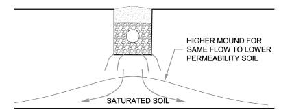
This is much the same with a water table below the dispersal area, the applied water will mound up to overcome the resistance of the saturated soil below the water table to sideways movement of the water.
