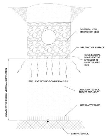
This capillary fringe is most saturated near the water table, and less saturated higher up.
