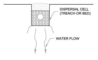
If the dispersal cell is located above a very low permeability layer, the water has to move to horizontally (sideways) to get out from underneath the dispersal area.
