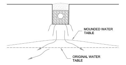
On a sloping site, the head pressure comes from a combination of the slope and the mound, and so the mound will be smaller as the slope gets steeper.
