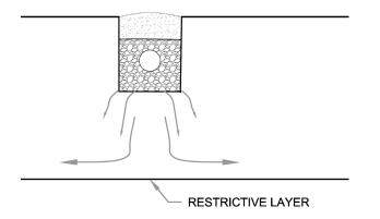
To move laterally, the water needs some head pressure to overcome the resistance to movement in the soil. On a flat site, this head can only come from the build up of a "mound" of groundwater under the dispersal area.
