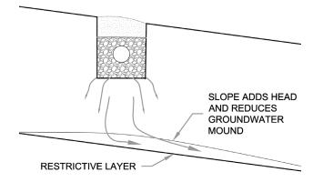
This groundwater mound continues to grow with time, and can reduce the VS below the system quite significantly. In many cases with poorly designed systems the mound will, over time, use up most of the VS.
