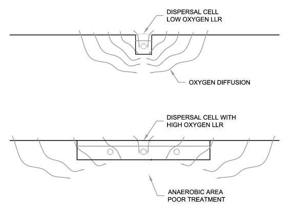
The maximum permitted effluent load per meter length of cell can be calculated. However, a simpler method was needed to address this and in BC we use two maximum LLR ranges to represent the "oxygen LLR" for a system.
