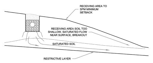
The capillary fringe is a problem here too—even if the water is near the surface contaminated water may wick up and cause a health hazard.
