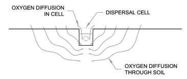
This oxygen has to diffuse through surrounding soil to get to the cell and to the soil below. This is not rapid; it is faster in dry soils and coarser soils. It is faster if the system is shallow so the oxygen has less distance to travel.
