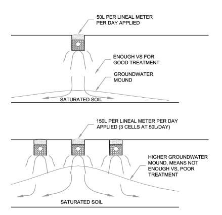
On a sloping site, the mound will be higher and also the amount of effluent flowing downhill per meter of contour length will be higher, and this may be too much for the available soil depth and head—resulting in breakout.
